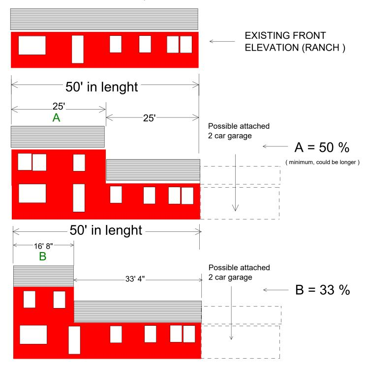
When converting 1 style house to another style house,in this case, ranch into a split level ranch, your objective (architectural-wise) is to make the finish appearance always look like this house was never converted..Usually the proposed upper level should be at least 50 % in length of the existing length of ranch, Any % less would look unusual, thus non-appealing. See examples above (A = appealing B = Non appealing)
